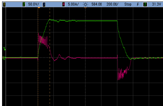
Figure 19. Current and Voltage Traces From Piezo IPhaseArray Configuration Example 1
